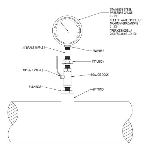
NOTE: 1. 2. ALL GAUGES TO BE GLYCOL FILLED AT A 4" MIN. ALL GAUGES MUST READ PRESSURE IN POUNDS PER SQUARE INCH (PSI) AND FEET OF WATER.
